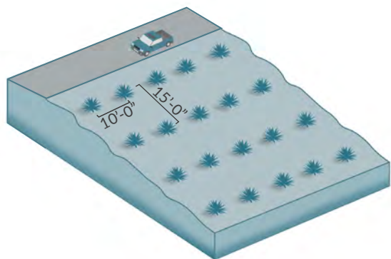
DIAGRAM: Spacing recommendations are dependent on the crop being planted. Top diagram shows basic fruit or deciduous tree spacing, bottom diagram shows spacing for succulents. Maintaining at least 10' between crops and 15' between rows helps reduce fuel loads.
