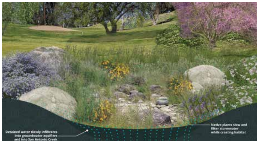
A large-scale rain garden planted with native trees, shrubs, and grasses that tolerate a range of soil saturations. Plants that thrive in high saturated soils are planted at the bottom of the rain garden, while more saturation averse plants and trees are planted on the edges.
