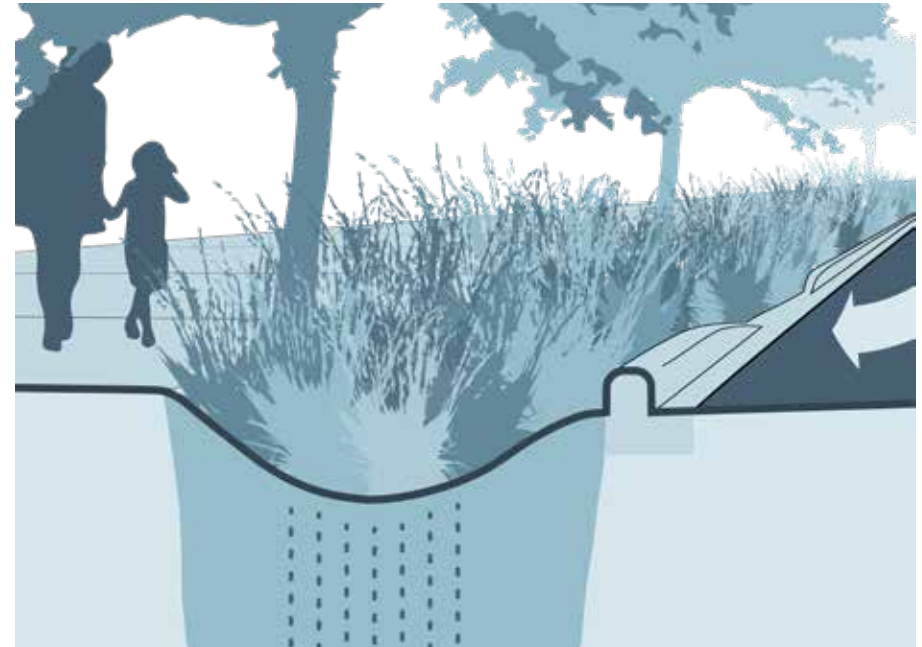
This image shows the infiltration effect on a Curb Cut basin. Basins should be planted with native plants that are adapted to intermittently dry creek channels and riparian areas. Source: Watershed Progressive
